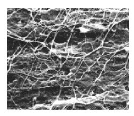
Structural reinforcement is created by the addition of **AP 101** fibers into the asphalt mix. In order to create the fiber network, **AP 101** needs a "carrier" into the liquid asphalt. The "carriers" of choice are called ThermoPlastic Elastomers or **TPE**'s for short.
